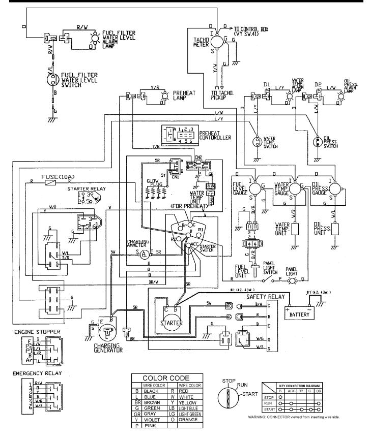
Figure 62. Engine Wiring Diagram
